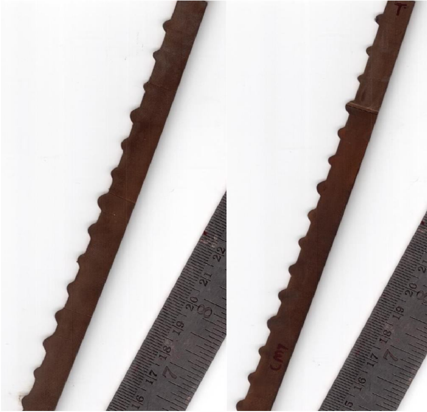
Figure 3.3 Cross section profiles of CMT and Pulse beads
