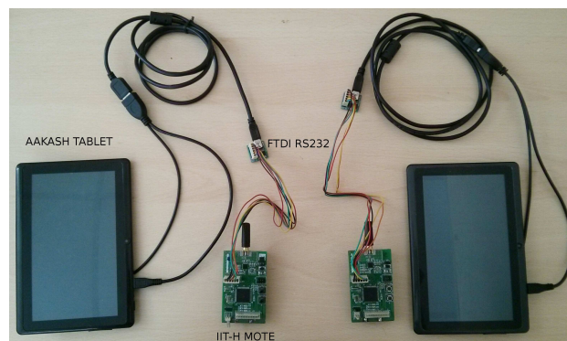
Fig. 2: Text messaging between two android devices (Aakash tablet) through IIT-H motes
