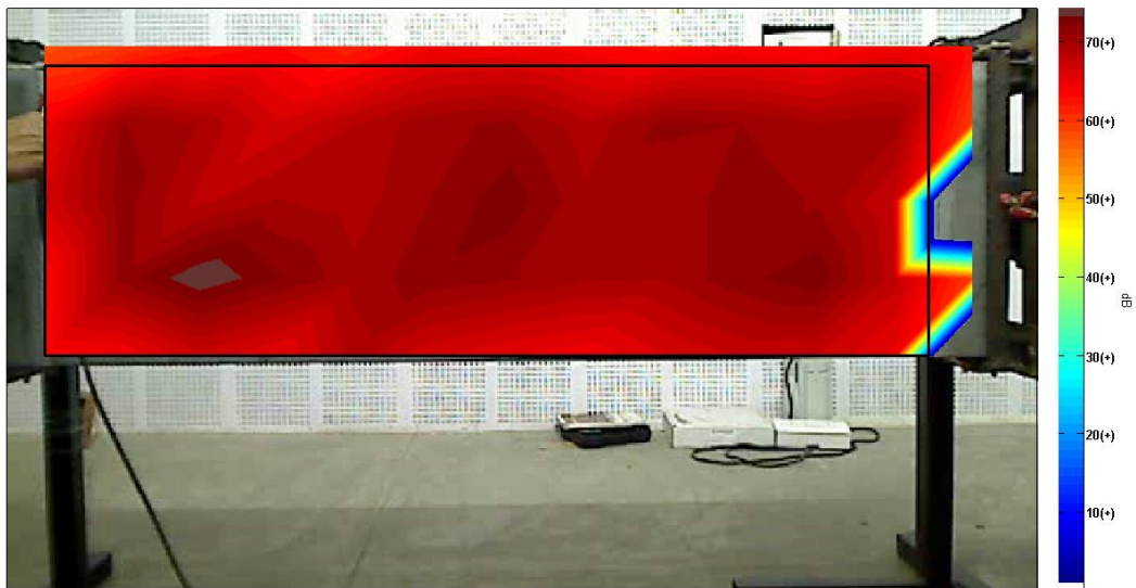
Figure 4.7: Generation of intensity colour plot after scanning duct surface
