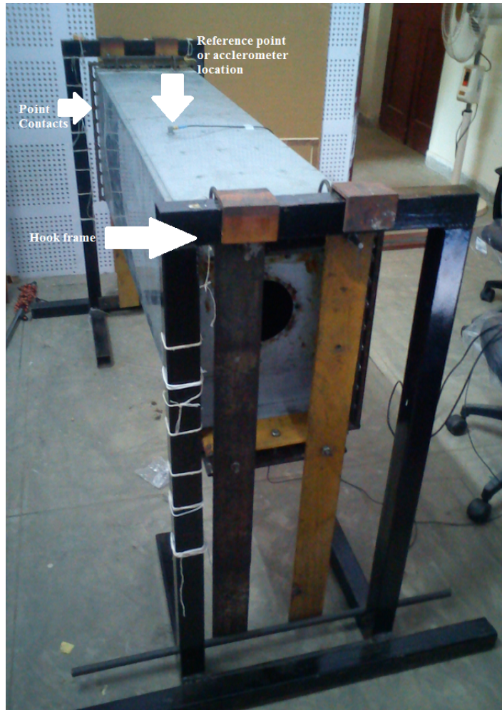
Figure 3.13: Rectangular duct(SS) for EMA set up
