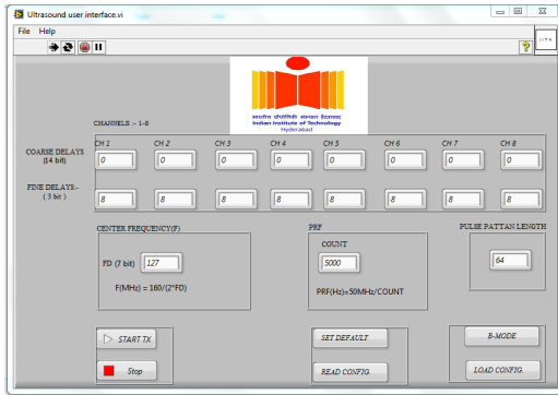
Fig. 7: User interface to control the transmission parameters
