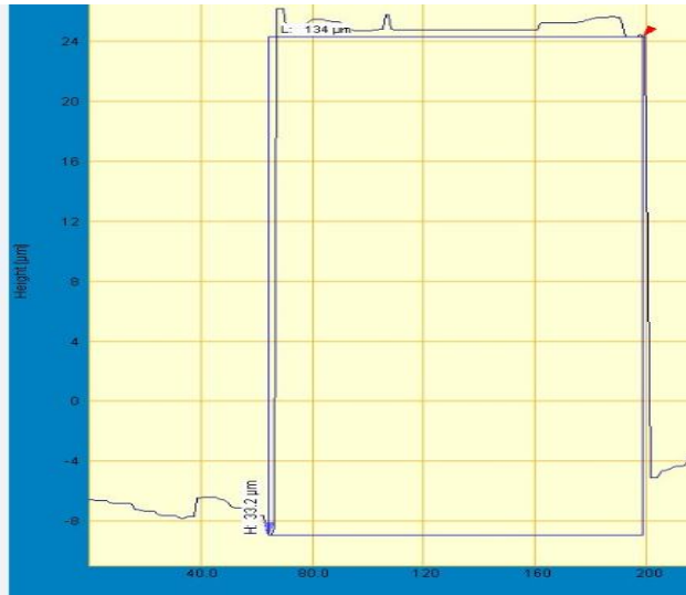
Fig. 5.6: Height and width of the etched pillar after first etching step.
