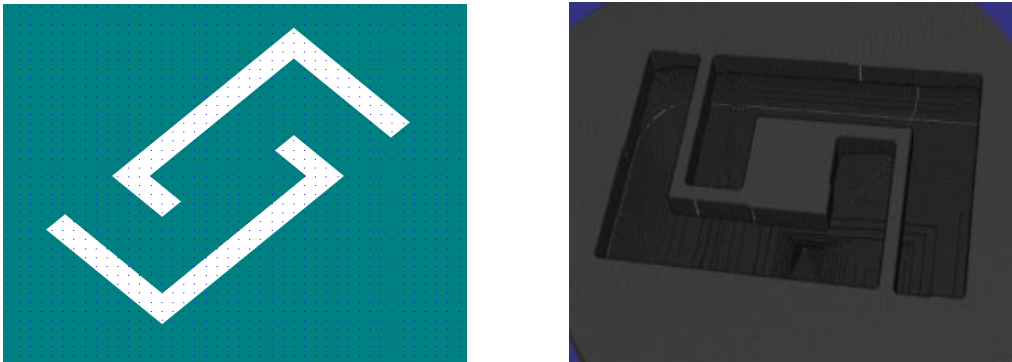
Fig.7.8: showing the mask used and the bolometer sensor membrane obtained using Intellisuite based FABsim physical simulation
