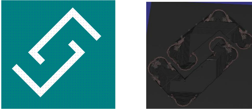
Fig.7.3: showing the mask used and the bolometer sensor membrane obtained using Intellisuite based FABSIm physical simulation.
