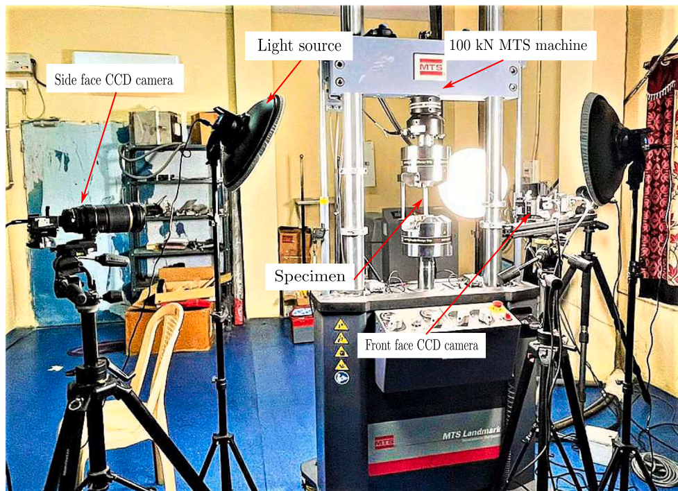
Fig. 5. Experimental setup for the tensile testing of the adhesive bonded scarf jointed CFRP specimen.
