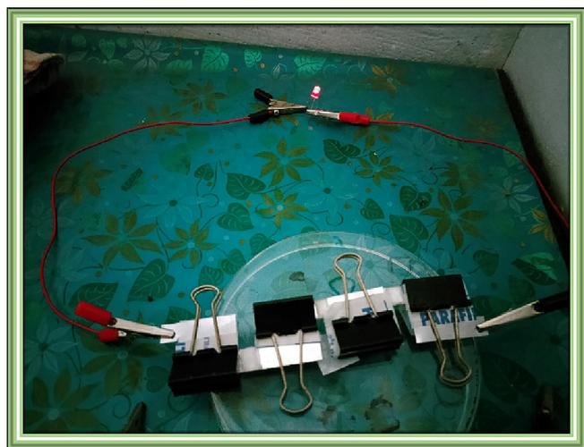
Fig. 13. The fabricated supercapacitors are energizing red light-emitting diodes. (For interpretation of the references to colour in this figure legend, the reader is referred to the web version of this article.)
