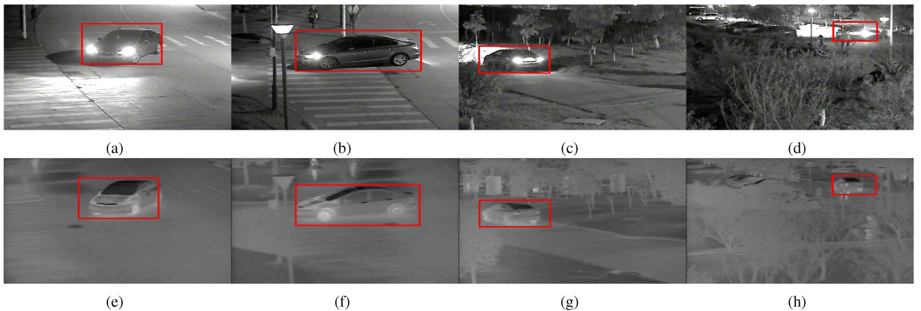
Fig. 3. Tracking results for VOT2020 dataset [53] with moving car target in sequential frames of RGB and thermal videos. (a)–(d) Output of the network for RGB images. (e)–(h) Output of the same CNN for thermal images. In both the cases, track is consistent as observed.
