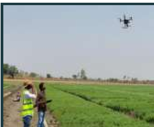
UAV Surveying to estimate canopy cover
