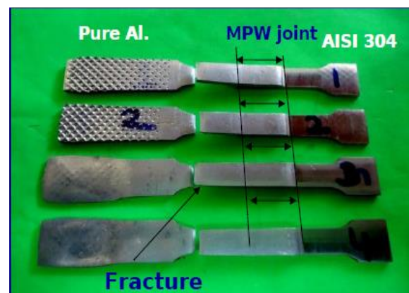
Figure 8. Lap-shear tests showing failure outside the welded zone.
