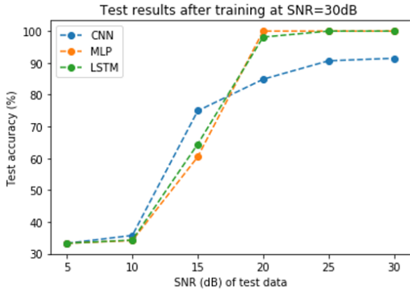
Fig. 1: Modulation classification performance of architectures in Table I in AWGN channel.
