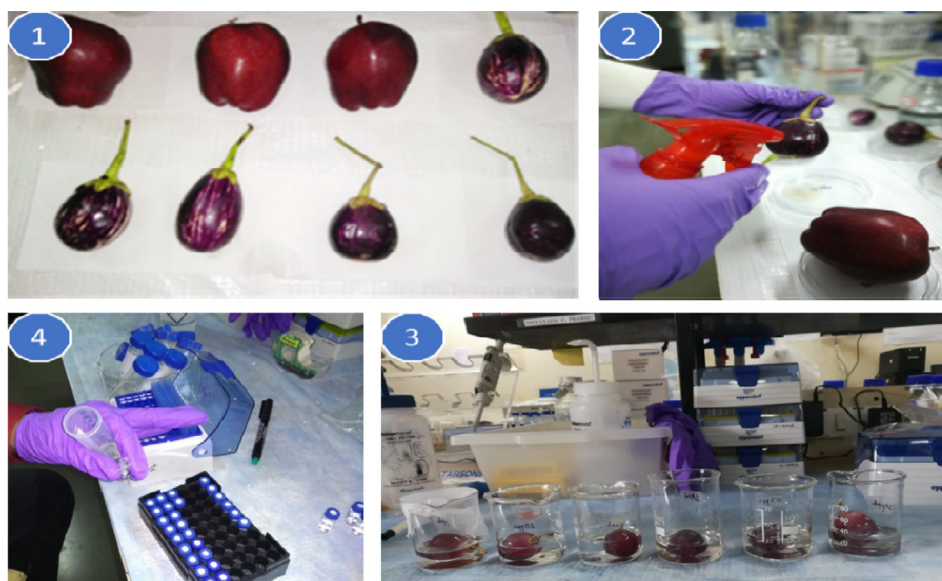
Fig. 5. Preparation of field collected samples towards parallel analysis using developed UIIS system and LC-MS instrument.
