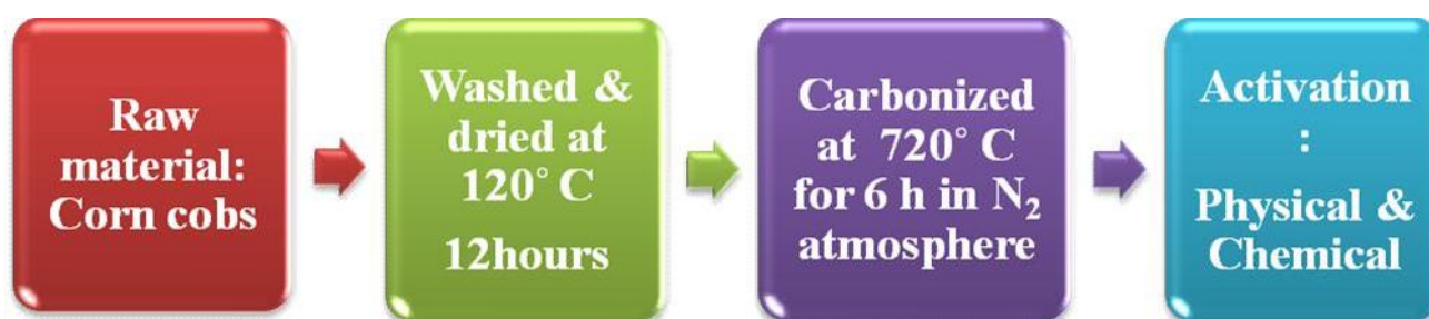
Figure 2. 2:Schematic representation for the preparation of activated carbon
